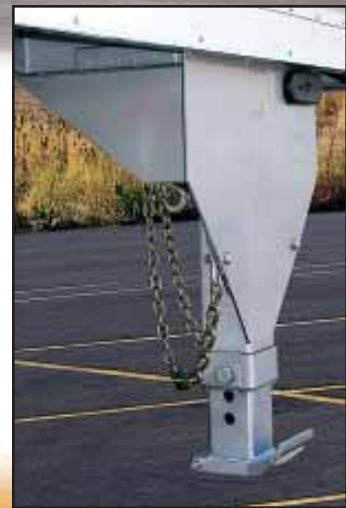
2 5 / 16 Adjustable Height Ball Hitch: Other hitch configurations available as optional equipment.
