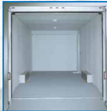
Standard Interior Floor and Sidewall Liner
