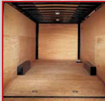
Standard Interior Floor and Sidewall Liner with optional D-Ring Tie-Downs
